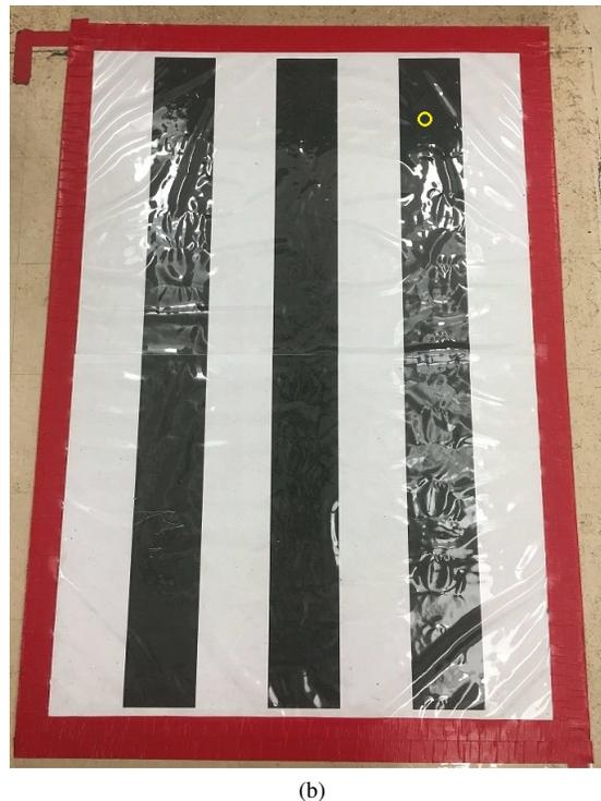
Fig. 1: (a) The scalar field with the ring pattern used in simulations. (b) The scalar field with the row pattern used in both simulations and physical experiments. The yellow circle on the top right marks the initial position for the robot.
