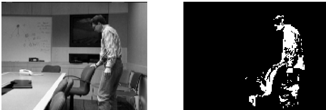
Figure 1: A video frame (left) and its segmented foreground (right). [6]
